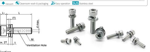
• The ventilation hole easily releases gas trapped in the screw holes of equipment and machines, and supports vacuum drawing of vacuum devices.
