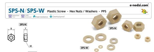
• Material/Finish RoHS2 Compliant SPS-N / SPS-W PPS (Polyphenylene Sulfide) / Bright Light Brown Main body Glass Fiber 40% Heat Resistance 200℃ Temperature\*1
